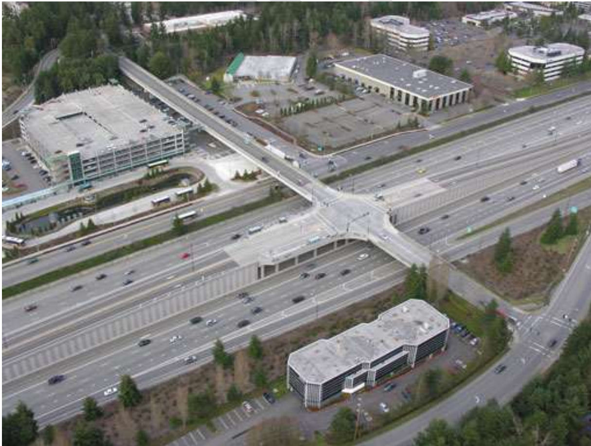
Figure 12.4.2 Aerial View of HOV Direct Access Ramps
