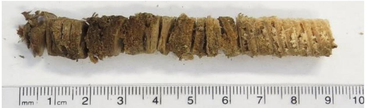
Figure 4.2.3.7 Wood Core Removed By an Increment Borer
