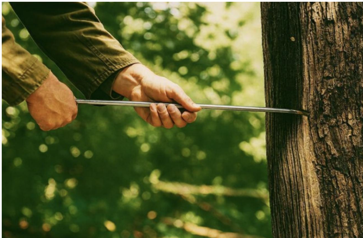
Figure 4.2.3.9 Use of a Shell Depth Indicator
