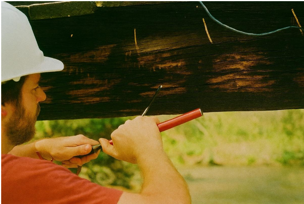
Figure 4.2.3.6 Simple Application of the Boring Tool
