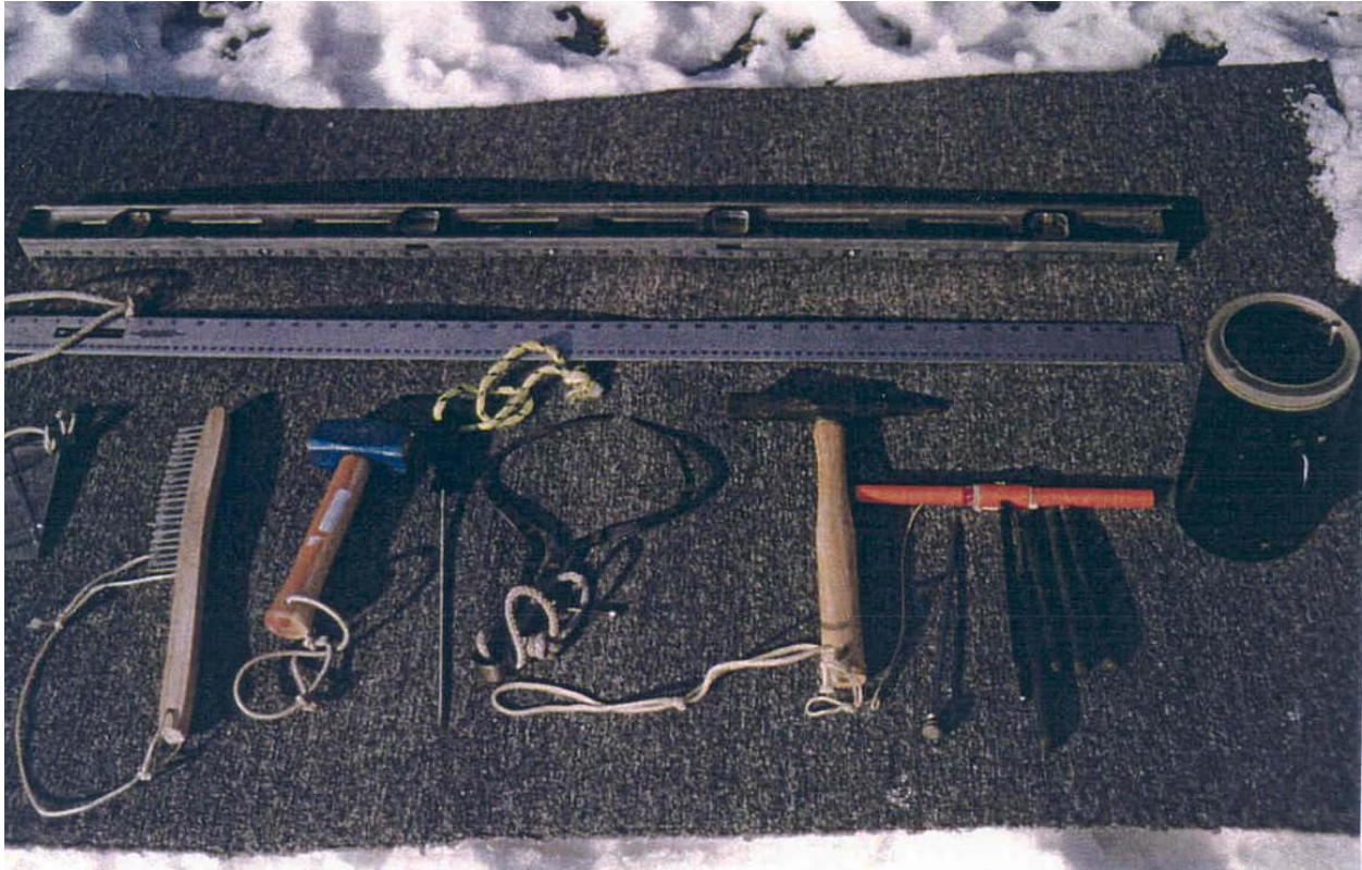
Figure 5.2.1.1 Typical Hand Tools for Underwater Inspections
