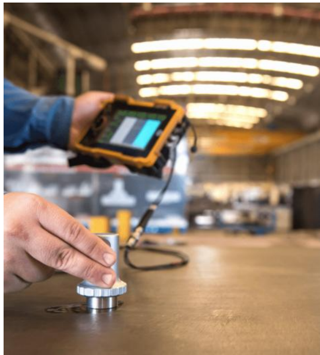
Figure 4.1.1.7 Application of Ultrasonic Testing Equipment
