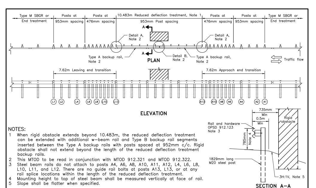
A Mounting height to top of steel beam rail shall be measured vertically at face of rail.
