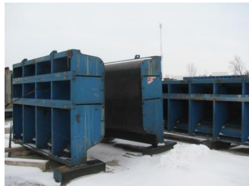
Figure 30 – NU Girder Forms
