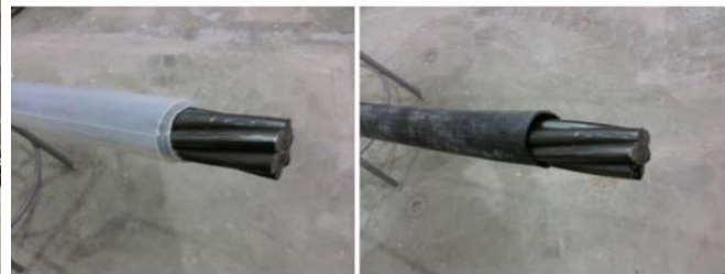
Figure 40 – Soft vs. Rigid Sheathing
