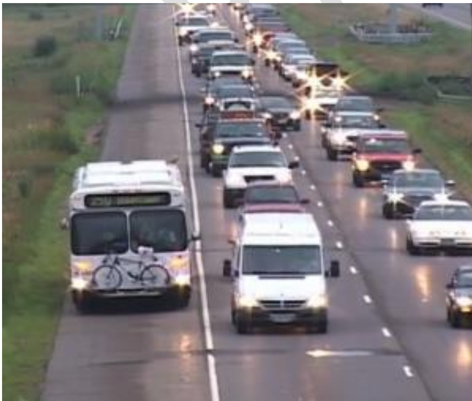
Figure 12.1.5 Bus on Shoulder in Minneapolis
