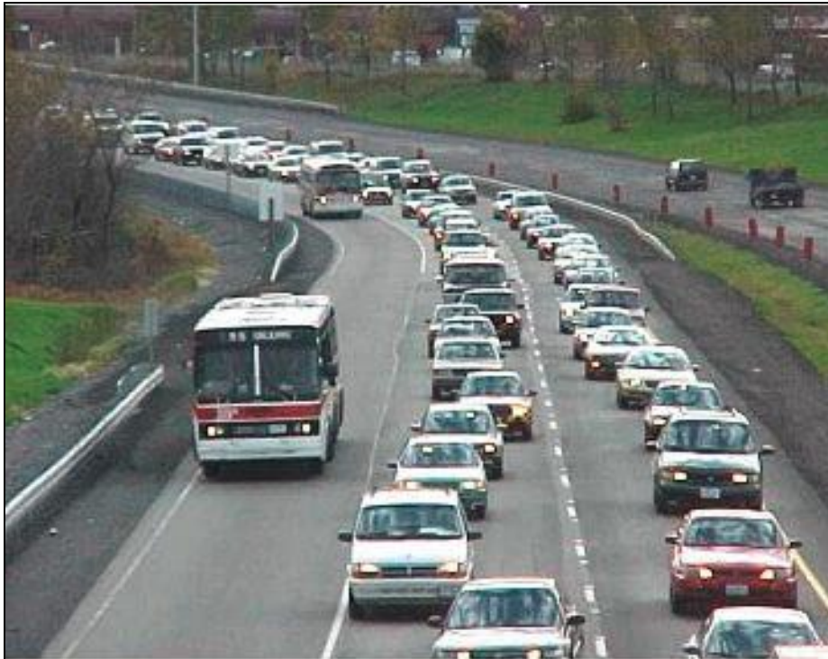
Figure 12.1.4 Bus on Freeway Right Shoulder (Ottawa)
