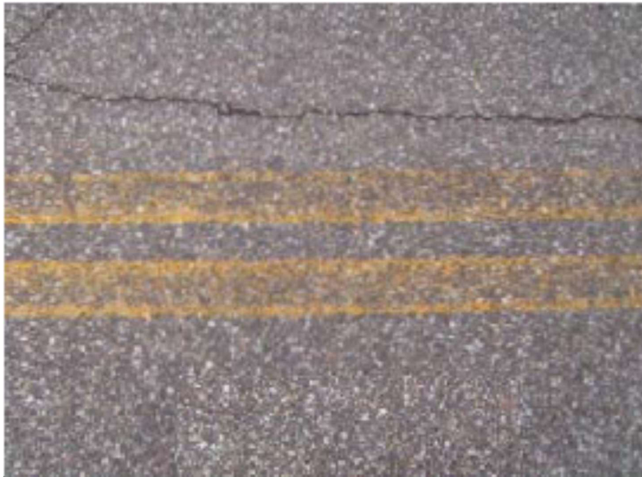
FIGURE 4: Durability Class 4 (75% to 85% Material Loss)
