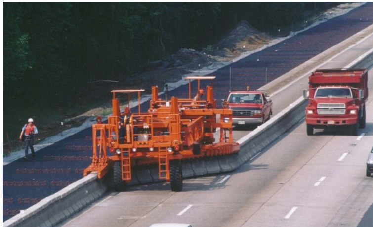
Figure 5-68: Quickchange Moveable Barrier Transfer Machine Shifting QMB Barrier
