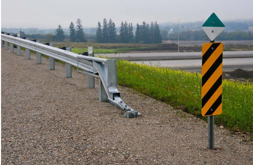
Figure 4- 2327 : SoftStop Terminal System
