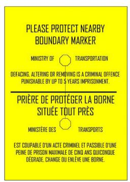
A marker post shall consist of a 1" sq galvanized tube delineator post x 7' long together with a yellow 7" x 9.5" polyethylene plaque as shown below. Plaque must be securely attached to the post using two 1/8" diameter 0.313" - 0.375" grip range stainless steel rivets and two # 5 0.140" x 0.438 " stainless steel flat washers.
