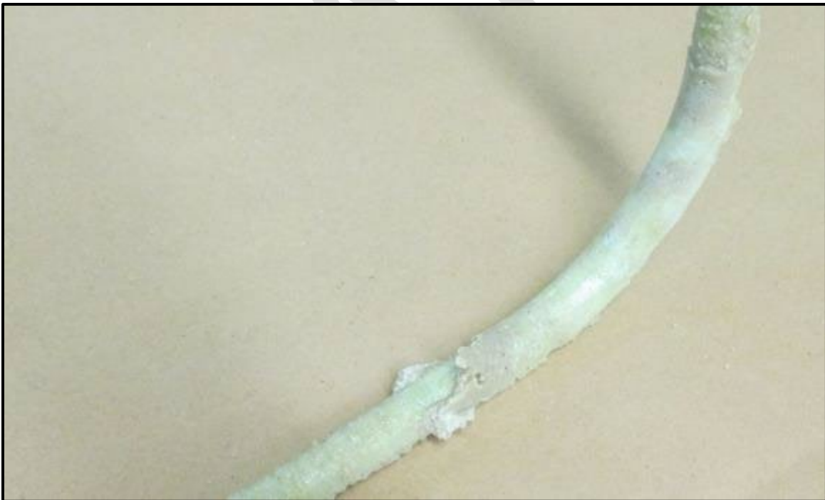
Figure 96 – Resin accumulation at the start/end of bend larger than 4mm (may be repaired by the manufacturer)
