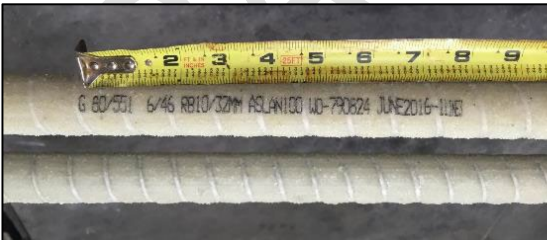
Figure 28 – Legible bar marking.
