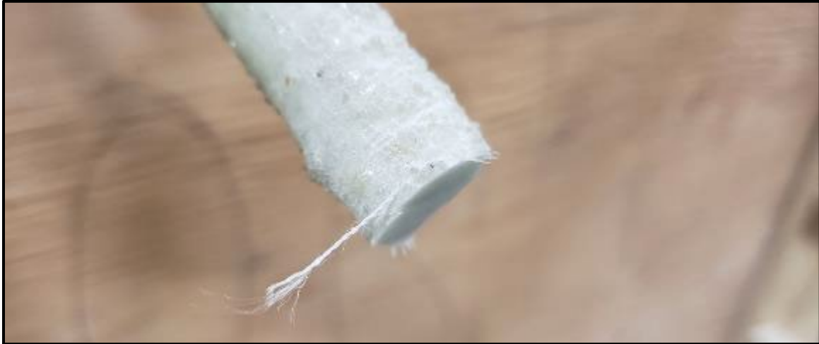
Figure 39 – Detached nylon strand
