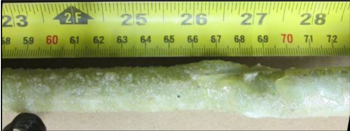
Figure 99 – Mis-aligned tooling print into the bend
