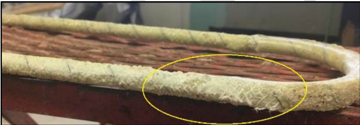
Figure 106 – Exposed fibres at bend
