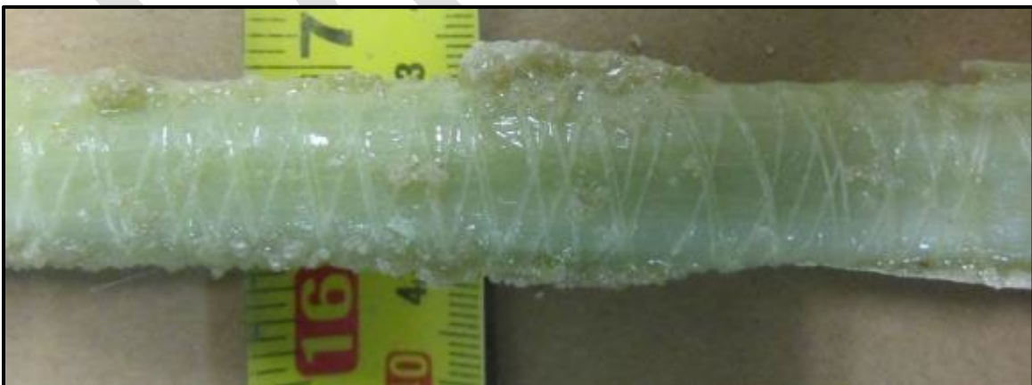
Figure 36 – 4mm resin accumulation
