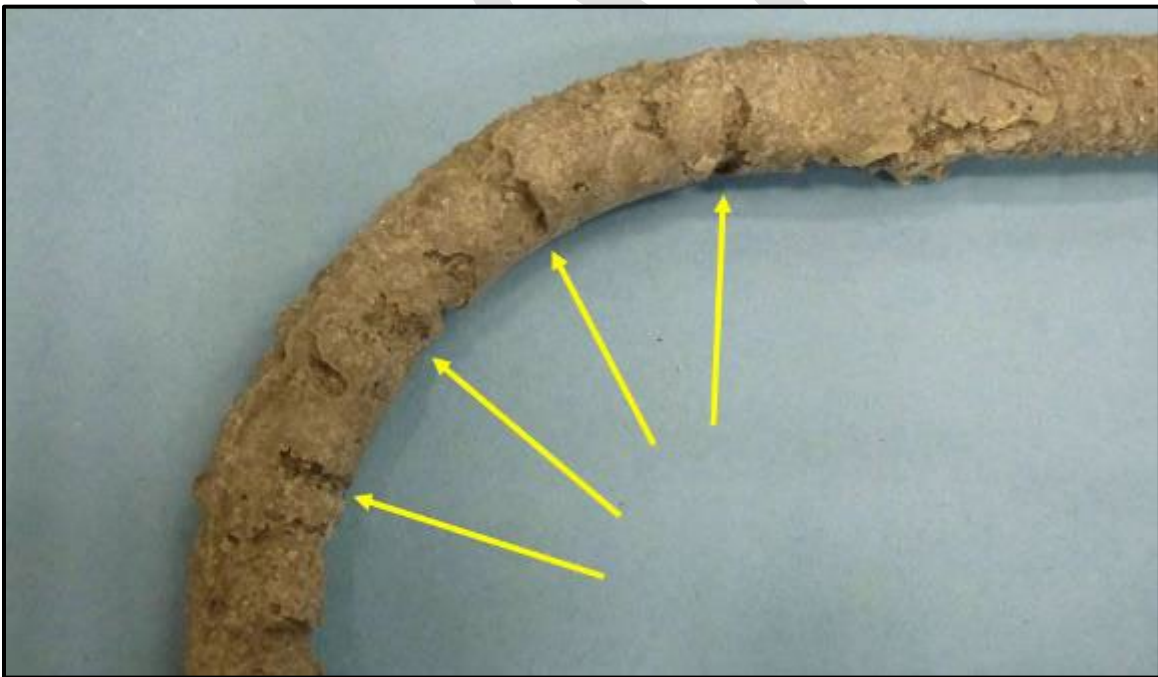
Figure 109 – Rejectable bar, with arrows pointing to surface voids
