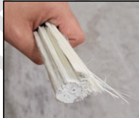
Figure 76 – Cut bar with frayed ends
