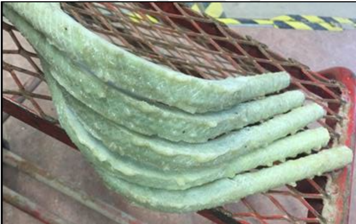
Figure 102 – Resin inconsistency (drips and runs)
