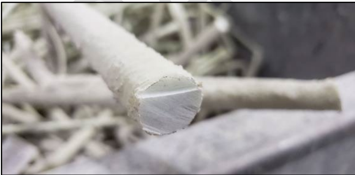
Figure 40 – Irregularly cut bar end
