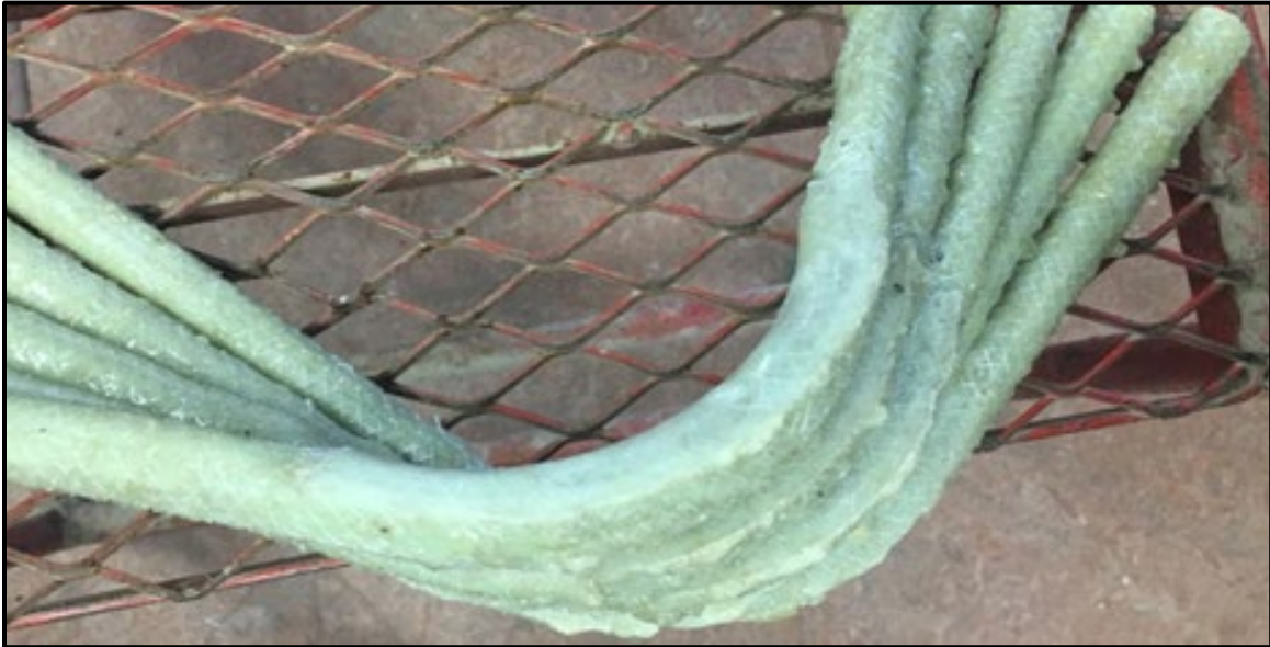
Figure 103 – Resin build-up on outer circumference of bend
