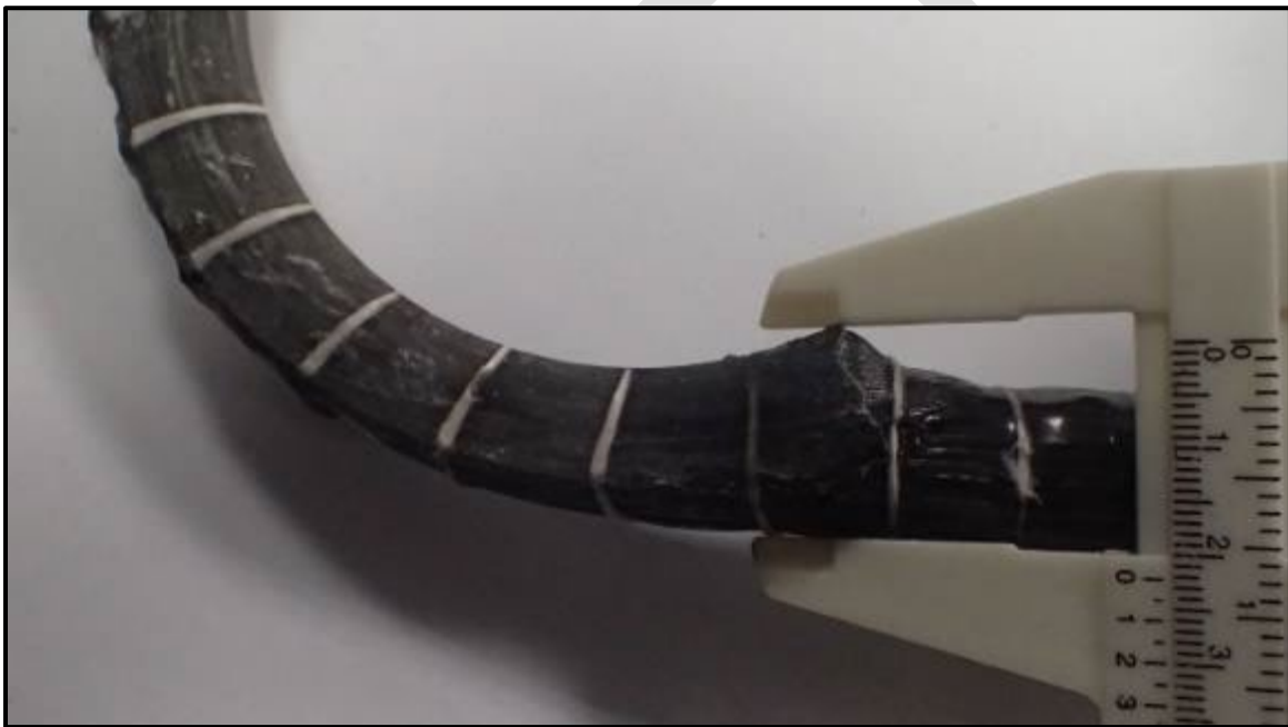
Figure 100 – Bend bulge more than the lesser of 4mm or 25% of diameter (17mm bar shown)
