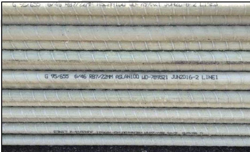
Figure 14 – Aslan GFRP manufactured by Hughes Brothers, Inc. (June 2016)
