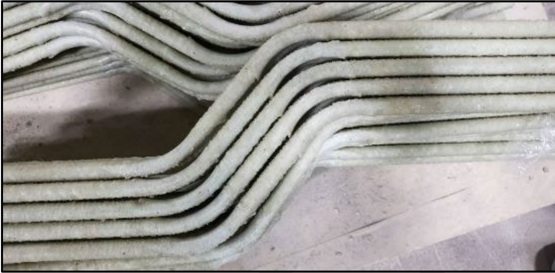
Figure 25 – Concave-convex bend sequence
