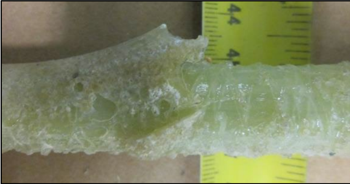
Figure 95 – Resin accumulation at the start/end of bend larger than 4mm (may be repaired by the manufacturer)
