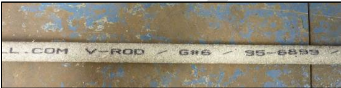
Figure 27 – Legible bar marking.
