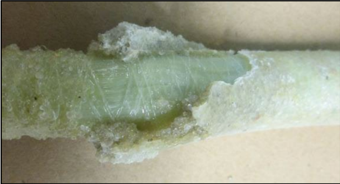
Figure 97 – Resin accumulation at the start/end of bend larger than 4mm (may be repaired by the manufacturer)
