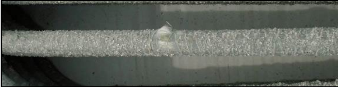
Figure 70 – Exposed and frayed glass fibres
