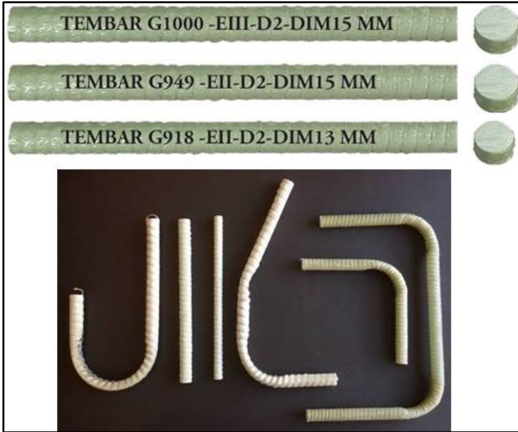
Figure 13 – Tembar manufactured by TemCorp Industries Ltd. (January 2018)
