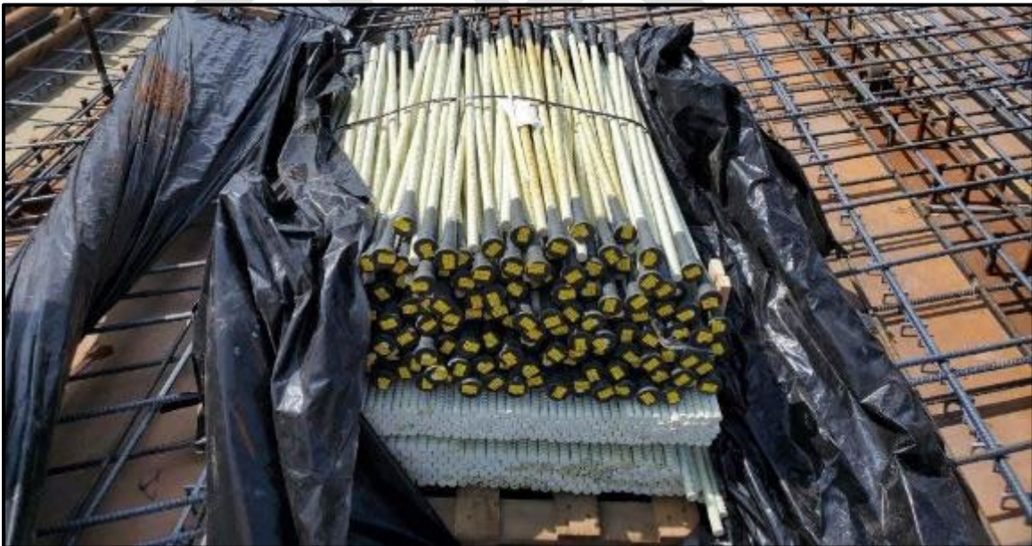
Figure 87 – UV exposure discolouration
