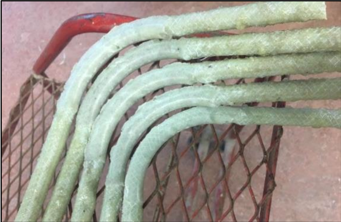
Figure 101 – Resin build-up and inconsistencies
