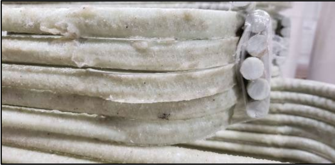
Figure 23 – Outside of bend
