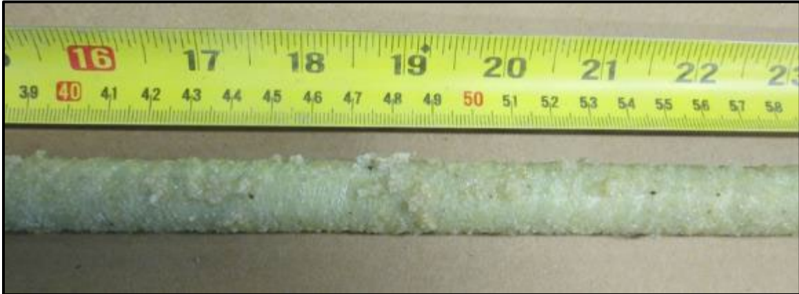
Figure 37 – Random resin accumulations
