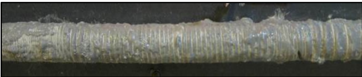
Figure 69 – Inconsistent resin coating and exposed fibres
