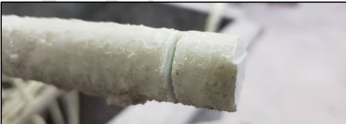
Figure 77 – Deep cut in rejectable bar
