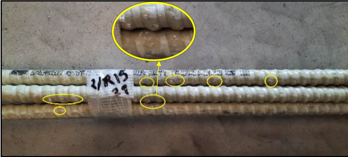
Figure 63 – Straight bar with voids/air pockets
