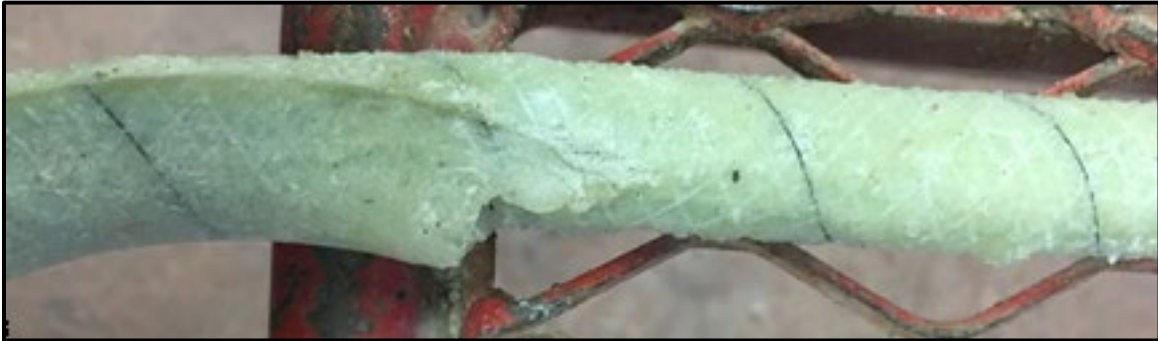
Figure 105 – Resin build-up at bend
