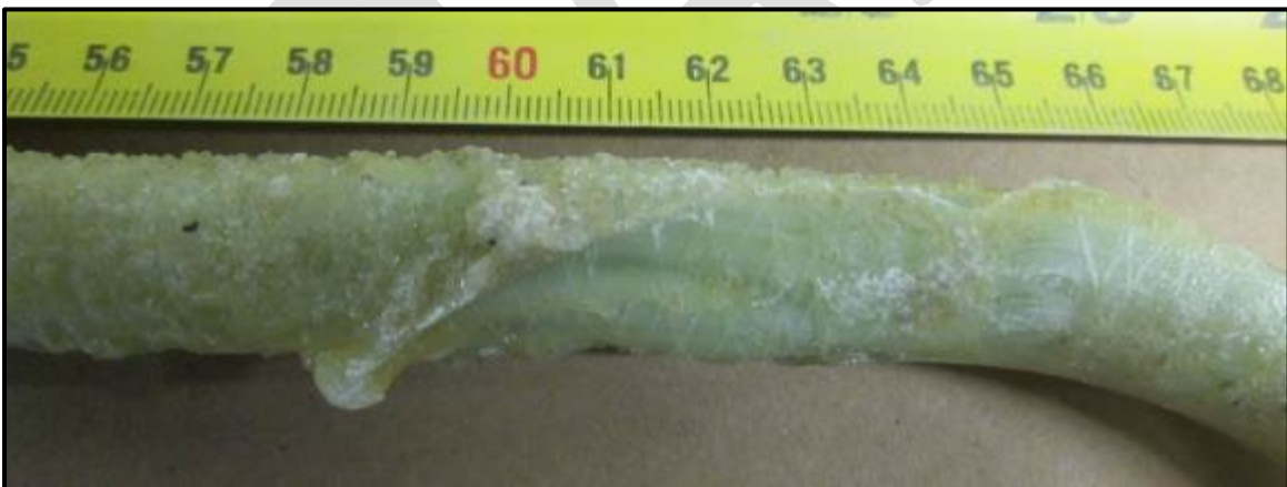
Figure 98 – Mis-aligned tooling print into the bend
