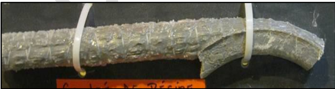
Figure 62 – Non-homogeneous resin distribution
