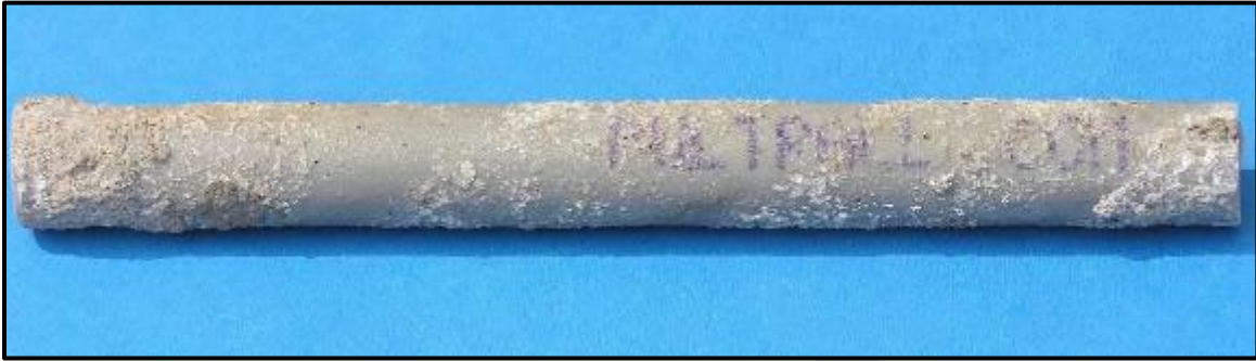
Figure 58 – Non-uniform sand coating
