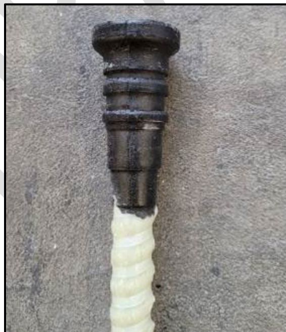
Figure 3 – MST-BAR: straight bar with anchor head
