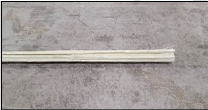
Figure 75 – Cut bar with frayed ends
