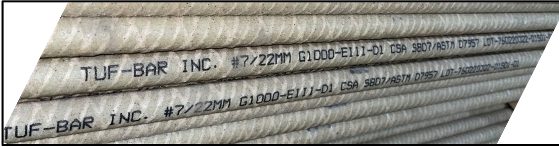
Figure 29 – Legible Bar Marking
