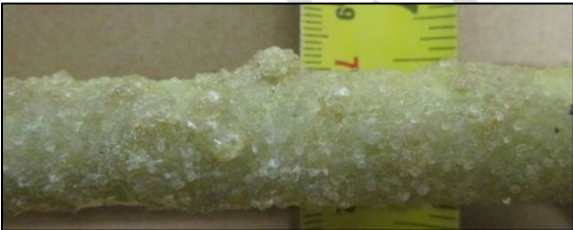
Figure 35 – 3mm resin accumulation
