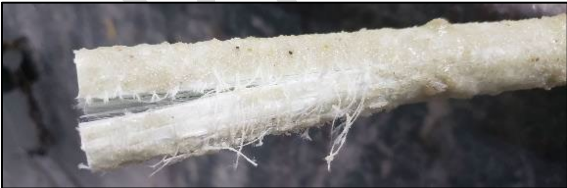
Figure 73 – Rejectable split bar
