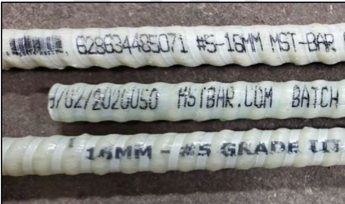
Figure 26 – Straight bar with formed deformation finish
