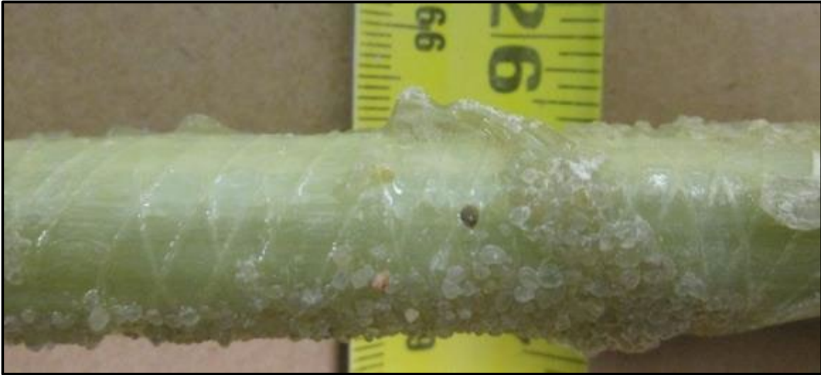
Figure 34 – 4mm resin accumulation
