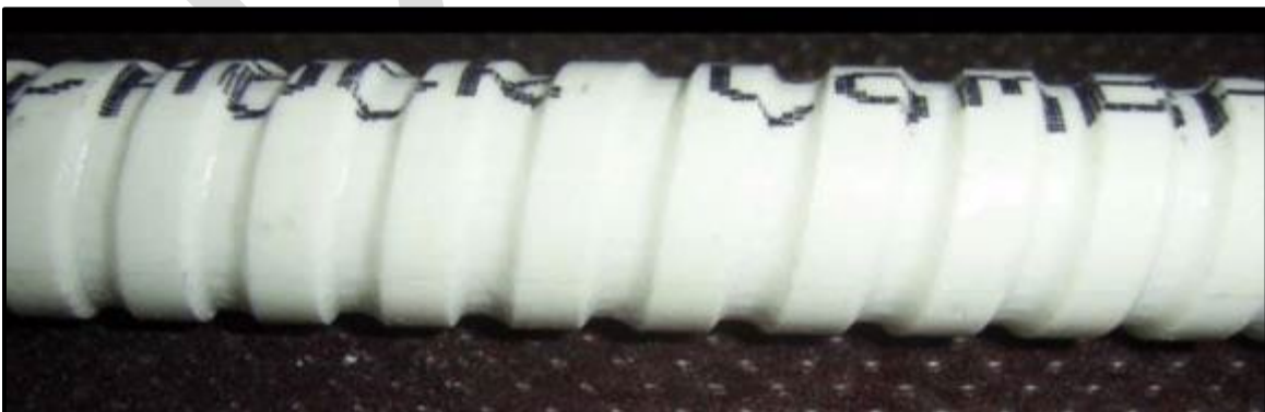
Figure 50 – Acceptable straight bar (Schöck ComBAR - Fiberline Composites Inc.)
