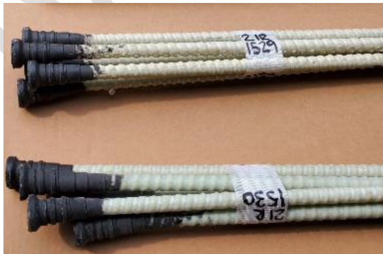
Figure 44 – Different coloured headed bars from the same production lot
