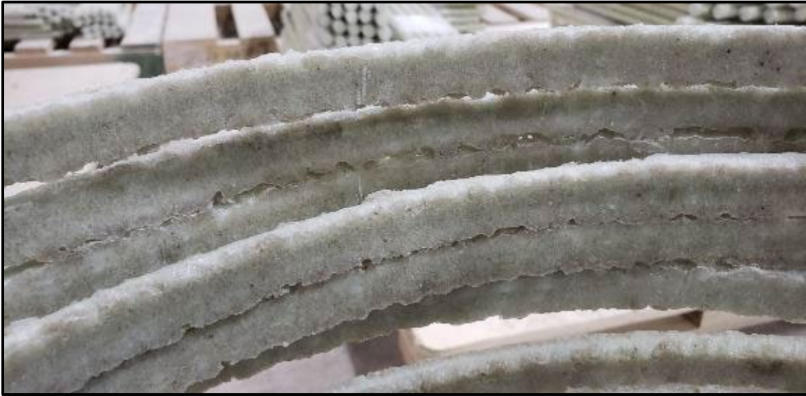
Figure 32 – Typical spiral with uniform, flat surface on inside of bend
