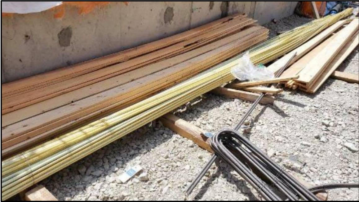
Figure 86 – UV exposure discolouration
