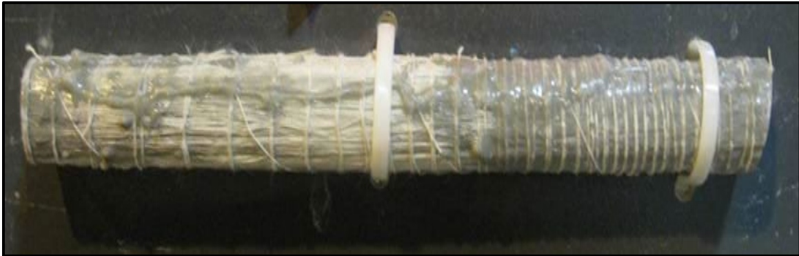
Figure 65 – Exposed glass fibres and inconsistent resin
