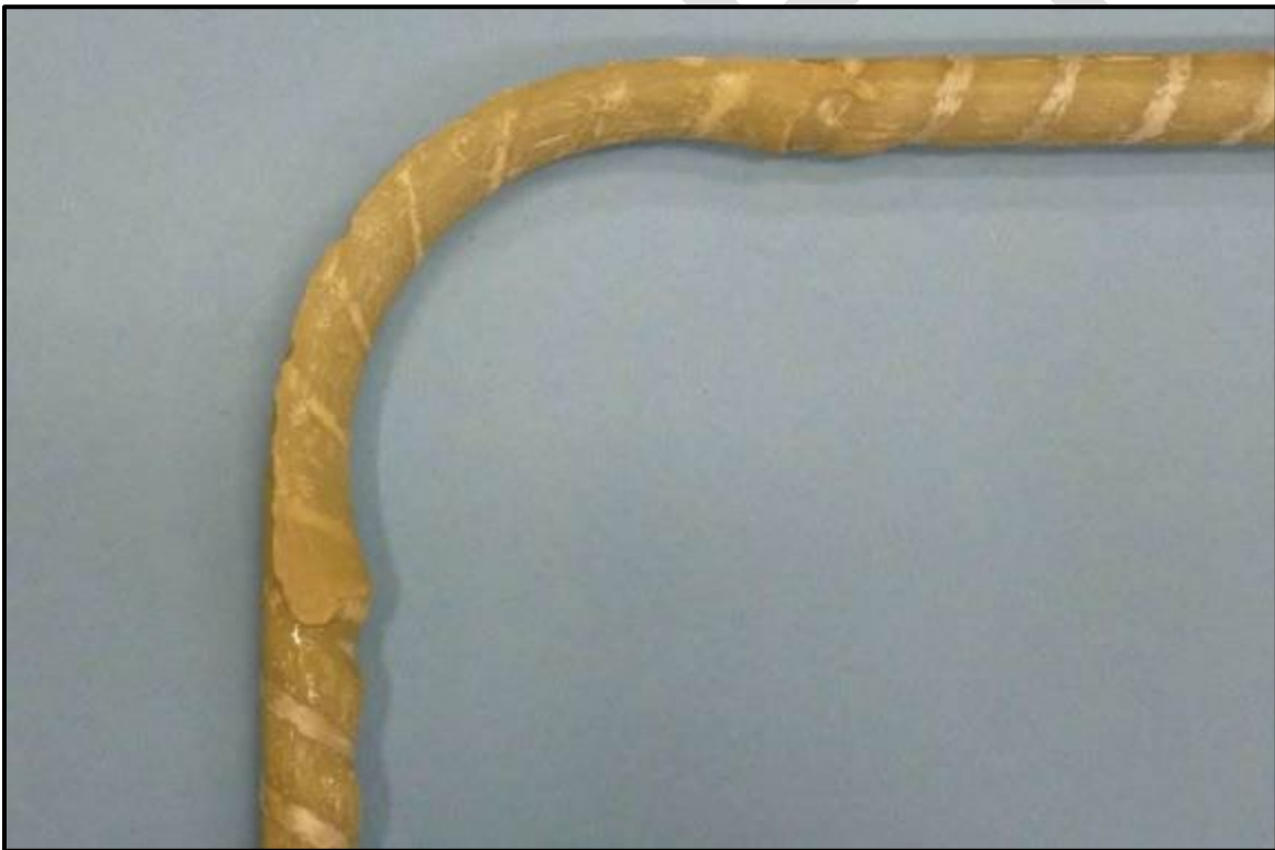
Figure 52 – Acceptable L bar with resin bulge. (Aslan - Hughes Brothers Inc.)
